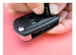
Start installing new pad by pushing one end of it under cut out of plastic shell, till it stays in place
