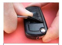
Start lifting corners of the pad, using screwdriver. Do not insert screwdriver inside the shell as you may damage electronic switches.
