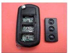
Prepare new Silicone Replacement Pad and wooden skewer for pressing new pad in. Do not use any sharp tools as you may damage pad or electronics.
