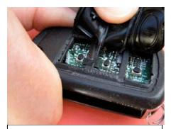
Middle part of the top cover needs to be pulled last so no rubber is left on the top of the shell.
