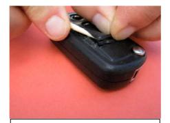
Continue the same process till last section of the new replacement pad engages with plastic cover.
