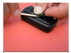
Continue the same process till middle section of the replacement pad engages with plastic cover.
