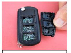
After removing top cover, your remote should look like on the picture above, with all electronic switches exposed
