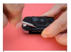
with flat screwdriver start lifting corners of the pad in shaving motion from both sides and ends of the cover.
