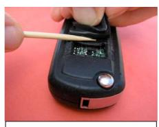
With help of wooden skewer, gently push new cover in till first catchers engage with plastic cover
