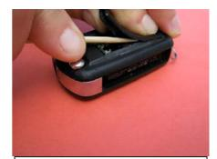
Continue pressing in with finger and help of skewer, till first section sits in cut out of plastic cover properly
